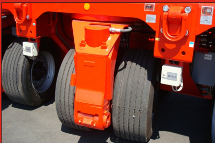
The new PST's feature 2 tires at 39" od and 16" wide with 192 psi.
